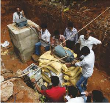
Block vibration test for dynamic soil properties
