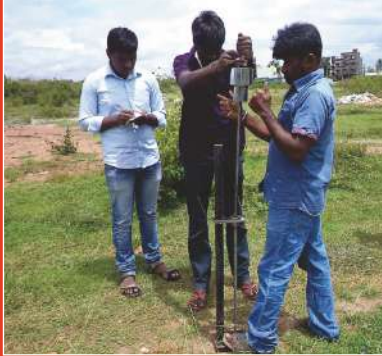
Penetration tests (SPT, DCPT, SCPT)
