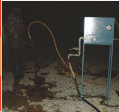
Field permeability test
